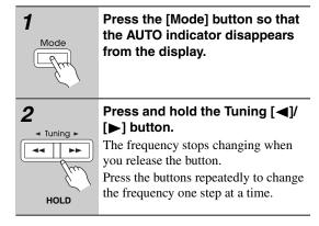
Radio Frequency can be changed in  $0.2~\mathrm{MHz}$  steps for FM and  $10~\mathrm{kHz}$  steps for AM.
